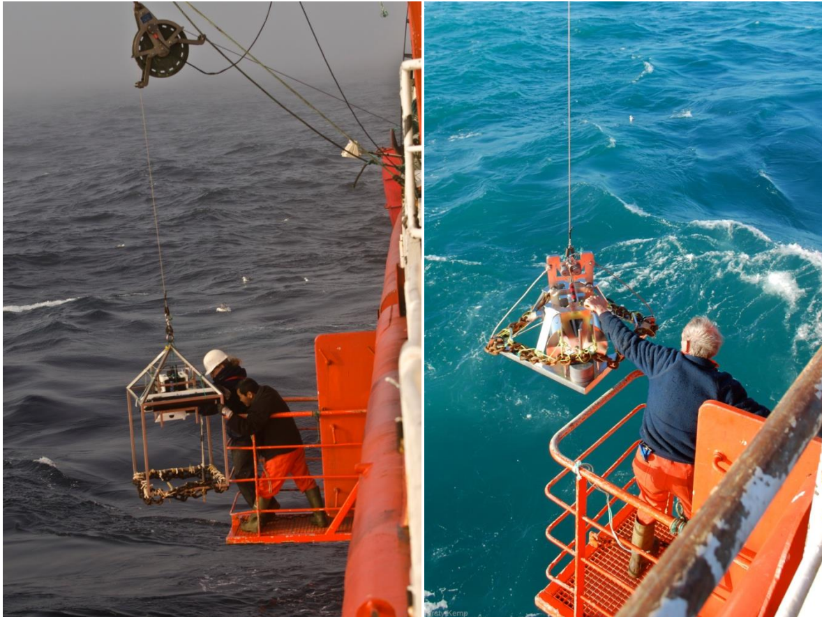
Figure 2. Benthic camera (image taken by Julius Nielsen) and Day grab in use
